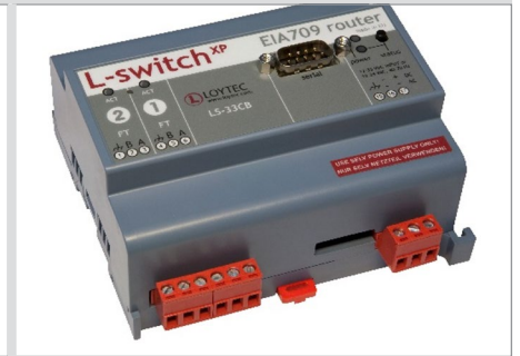
Figure 33. 1N-Lswitch: LonTalk router between two TP/FT-10 (media) network segments. This also has an RS-232 console port for configuration (generally not used).
